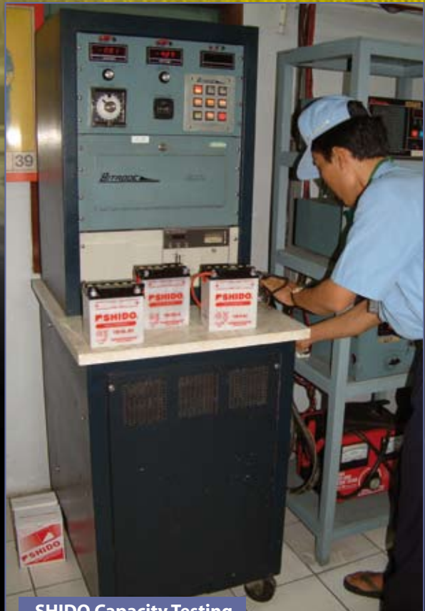
SHIDO Capacity Testing
